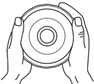
**Step 5:** Installing the motor. For first use, press the motor onto the collection tray. Make sure the **silicone ring** is properly attached to the **collection tray**.
